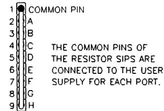
MODULE IS SHIPPED WITH ALL PULL-UP SIP RESISTORS INSTALLED
