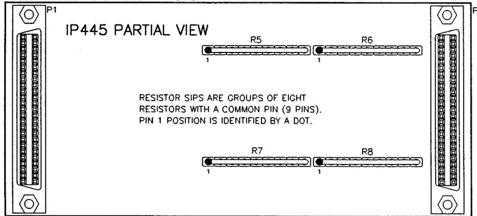
PULL-UP RESISTOR SIPS ARE MOUNTED IN SOCKETS AND CAN BE REMOVED IF REQUIRED. RESISTOR SIPS ARE DIVIDED AS SHOWN
