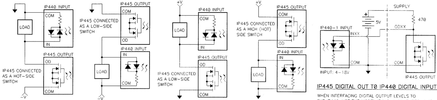
THE IP440 & IP445 INCLUDE 4 PORTS OF 8 CHANNELS EACH. EACH PORT SHARES A PORT COMMON. SEPARATE PORT COMMONS FACILITATE PORT TO PORT ISOLATION. THE IP445 ALSO INCLUDES SEPARATE PORT SUPPLY PINS FOR CONNECTING TO THE ON-BOARD PULLUPS.
