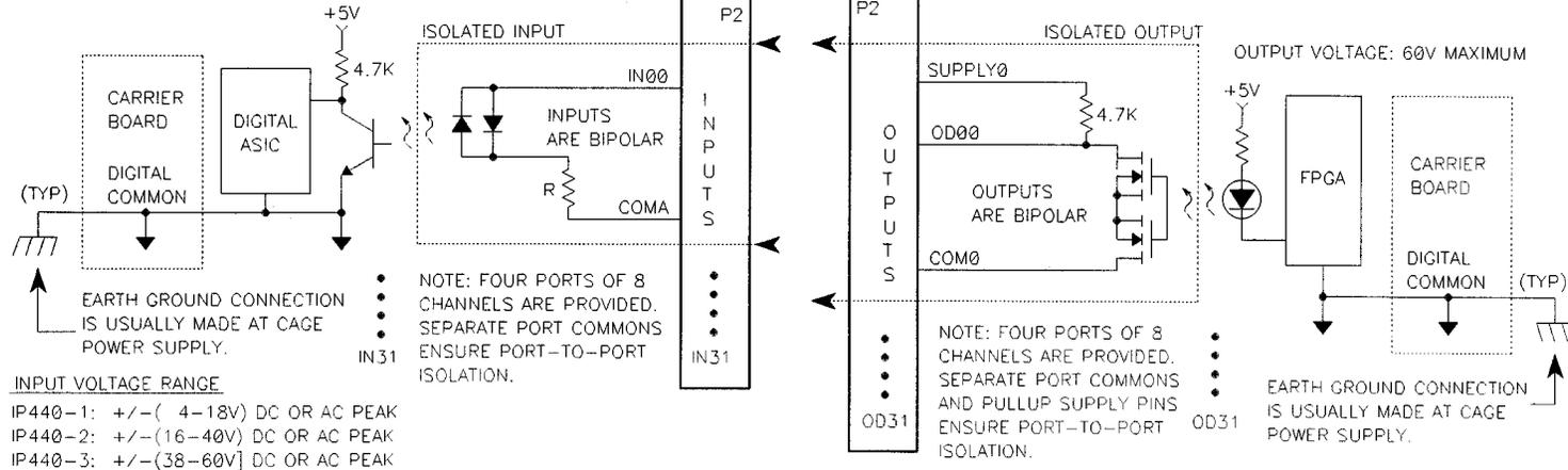
NOTE: FOUR PORTS OF 8 CHANNELS ARE PROVIDED. SEPARATE PORT COMMONS ENSURE PORT-TO-PORT ISOLATION.
