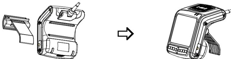
As shown in fig, insert the support bracket from the back of the instrument, place the instrument on a desktop; adjust the angle of the support bracket to adjust the screen visual angle.
