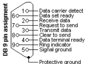
Used Pins: 2:TxD , 3:RxD and 5:Signal Ground
