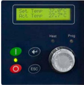
To control the system the controller has few “easy to use” buttons. Simply turn / press desired button. All information are displayed on a Liquid Crystal Display (LCD).
