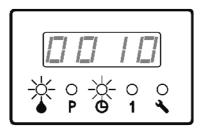
If PAUSE time is set as 0 (zero), LED monitor only displays "LUb" in LUBE state.
