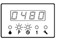
**4.** Press to confirm the new PAUSE parameter. LED now displays "LUb", which means the controller is now in LUBE time setup state.
