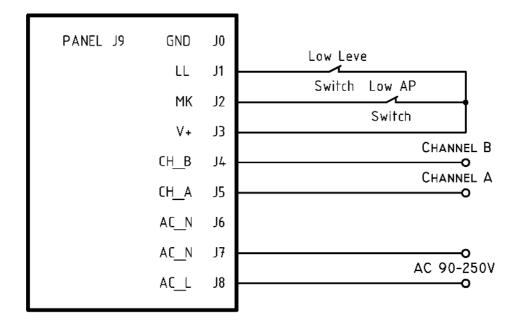
Channel A and B's outputs belong to live wire (AC\_L), their return current is on neutral wire (AC\_N). Lubrication devices should be connected between CH\_A and AC\_N, CH\_B and AC\_N.
