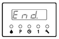
13. Press key **()**, controller then quit programming mode and back to normal operation display states. All the new programmed parameters will be saved permanently until next change via programming.
