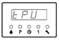
8. Press key 2 , light LUBE on. LED displays the current preset pulse time for channel A.
