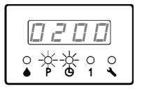
If controller is now in LUBE phase, and PAUSE is NOT set as 0 (zero), then LED monitor shows the LUBE remain value. **Example**: Current remain value of LUBE is 10s.
