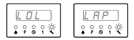
Left figure 'LOL' means Low Oil Level fault occurs.
