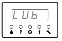
5. Press , light LUBE on, LED onitor displays preset LUBE time.
