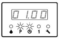
**12.** Press key **12** to confirm the new pulse interval time.
