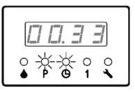
11. Use keys **C** to change pulse interval time value. **Example:** change to 1s.
