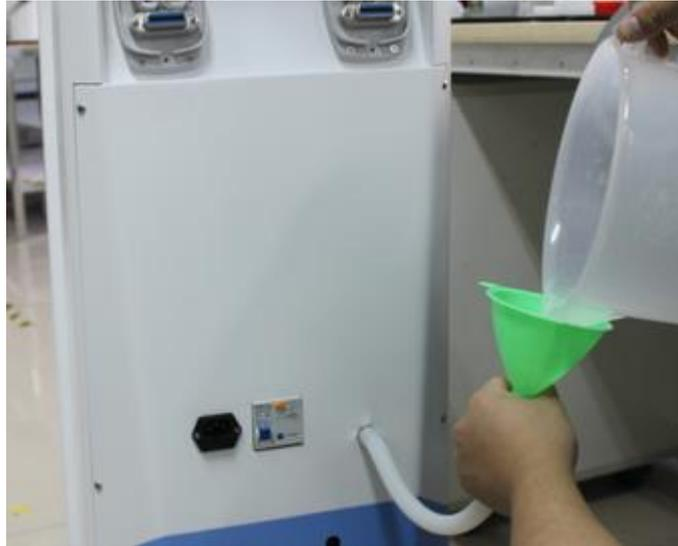
E. Fill in water until the overflow(vents) overflows, shows the water is enough. You can also observe by the water level viewing window.
