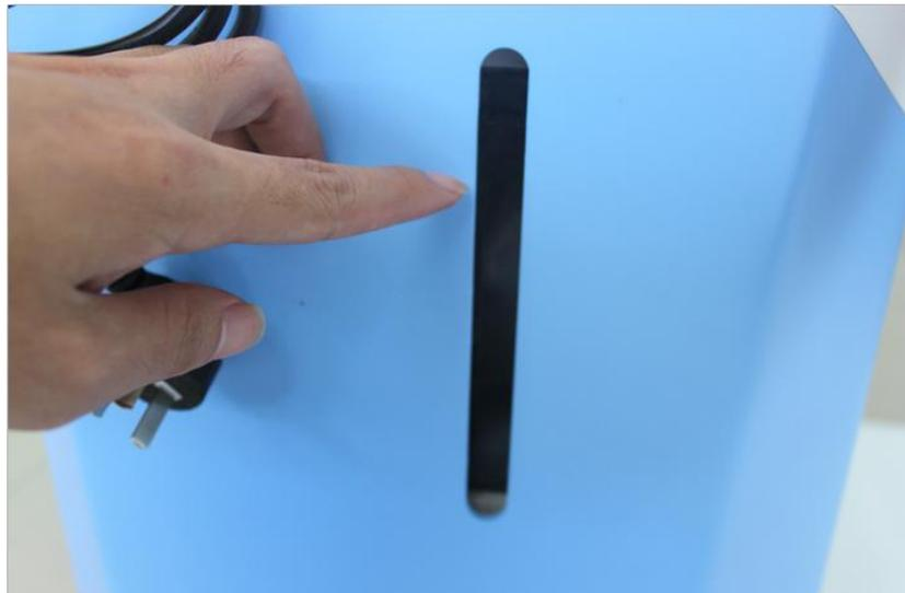
F. Do not tighten the overflow mouth at first, please wait until the machine finish debugging, then tighten the overflow mouth. The inside of the machine is a closed water loop, if tighten overflow mouth at first, there will be air inside the water tank,which will make water do not circulate, cause machine failure.
