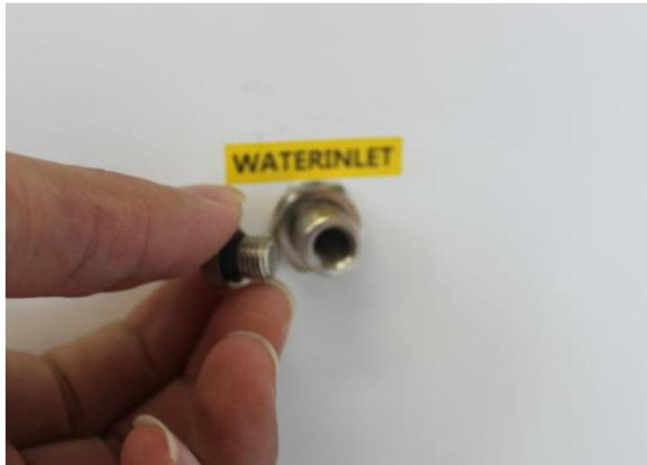
C Unscrew the overflow(vents) at he back of the machine. You can fill in water only when the overflow(vents) is open.
