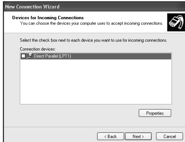
Figure 190 Selecting Devices for Incoming Connection
