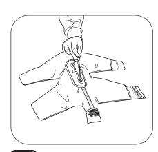
step 4 Pull tabs through the center opening of the Heat Exchanger and secure to the Cover.
