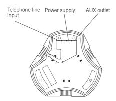
Connect cable 900102085 between the AUX outlet and the headset phone connection. Follow instructions in the headset manual to adjust levels.
