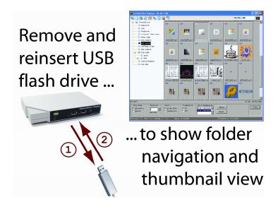
If your ShowBox is in Autoplay mode, you can change to Configuration/Thumbnail mode by simply removing the USB flash drive and plugging it back into the USB port on the front of the ShowBox chassis.
