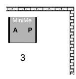
Fact: Subwoofers reproduce frequencies with wavelengths that are long in relation to the dimensions of most living rooms. Standing waves will boost or cancel various frequencies due to the interaction with the room boundaries. Moving a subwoofer in a room will change what you hear in the listening position a lot.
