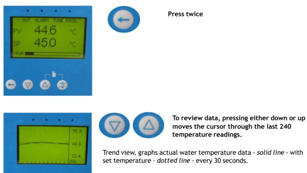
Trend scale adjusts automatically to actual water temperature data.
