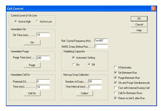
Taking drift issues into consideration, it is also a good idea to select the "cell on between runs" checkbox, to keep the crystal oscillating at all times.
