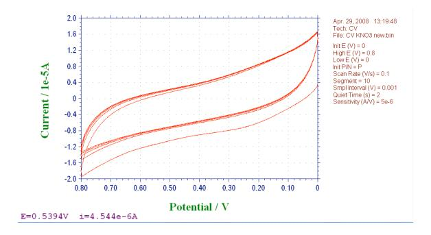
Containing 0.1M KNO<sub>3</sub> as well as 0.01M K[Fe(CN)<sub>6</sub>], this illustrates the oxidation and reduction of a solvated species (in this case  $Fe^{2+}/Fe^{3+}$ ) due to a varying potential
