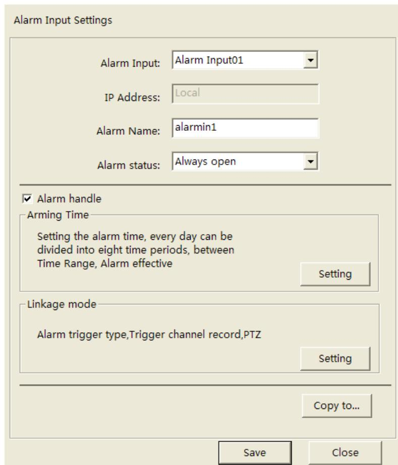
Step2: Select the type of alarm input, "NO" or "NC".
