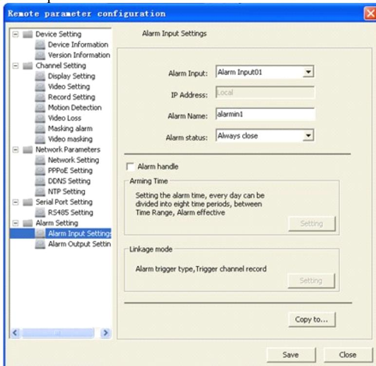
Step2: Select the type of alarm input, "NO" or "NC".
