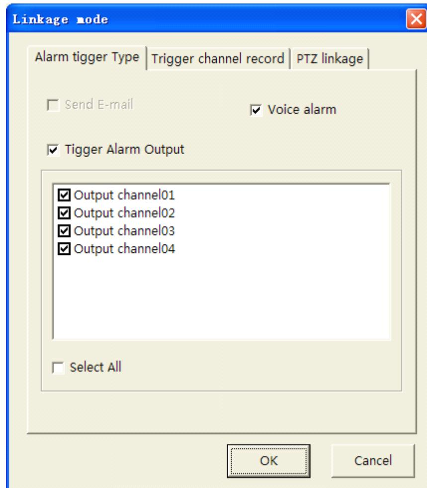
Step6: Set Trigger Recording for signal level alarm.
