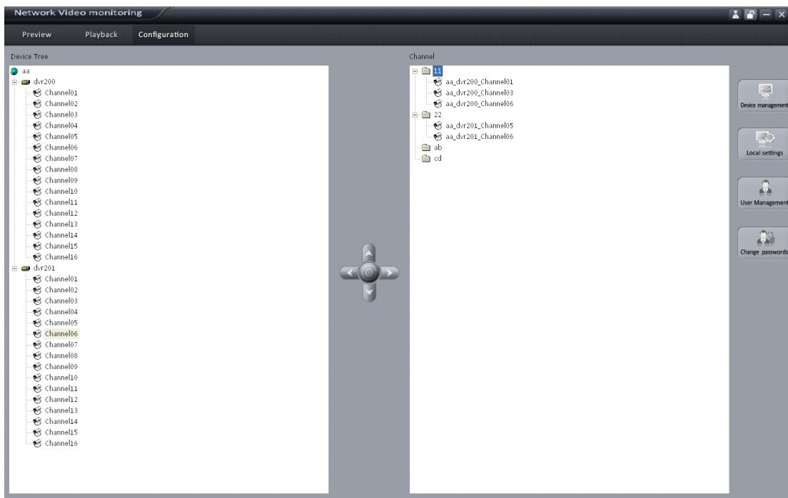
Select the device in the list area and click key and all the channels of the device can be moved to the selected group.
