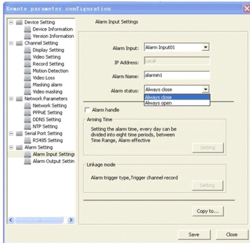
Step3: Enable "Alarm Handle" to activate "Arm Schedule" & "Linkage Method".
