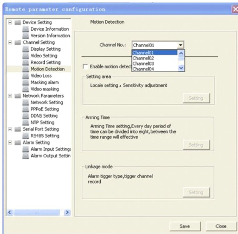
Step2: Enable motion detection to activate "Setting Area", "Arm Schedule" and "Linkage" settings.
