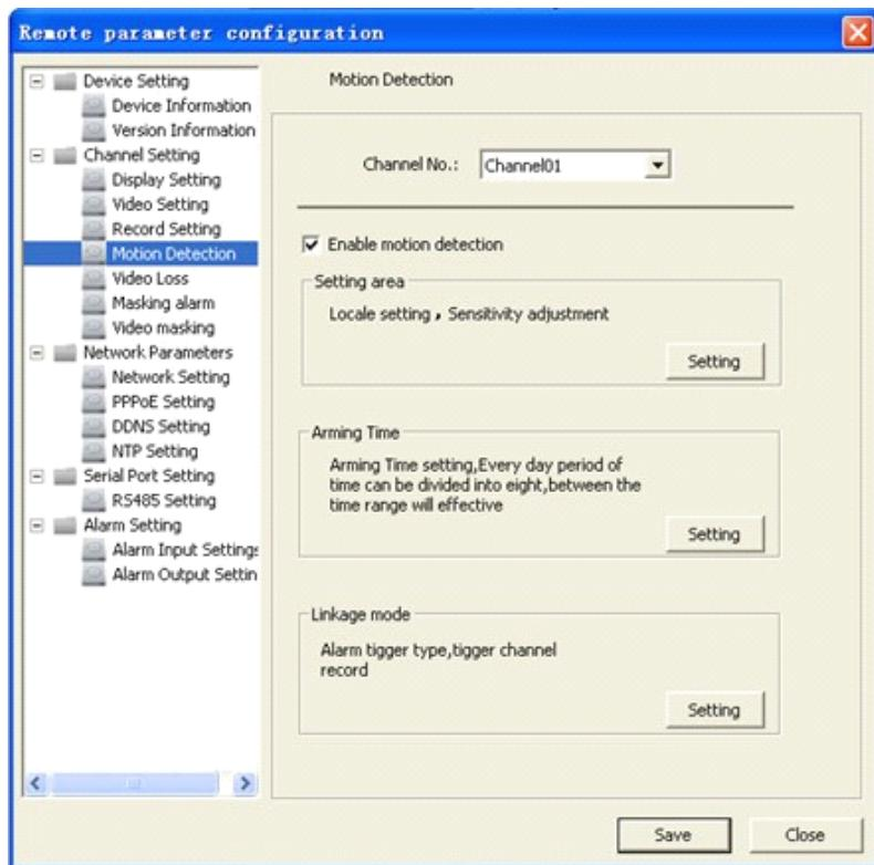
Step3: Set the motion detection area and sensitivity. Enable "Start Draw", and select the detection area by using mouse.
