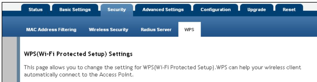
To use WPS function to set encrypted connection between this access point and WPS-enabled wireless client by WPS, click 'WPS Setting' in the web management menu, and the following information will be displayed:
