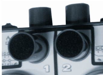
Figure 3-4: Filter at inlet of system
