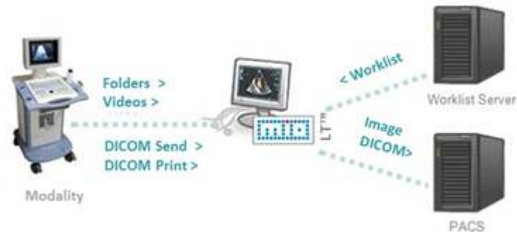
Figure 1.1: Basic scheme of MIO LT™ installation: image capture, reception of patient data and sending to PACS
