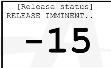
The display shows a countdown timer with the amount of time remaining before the extinguishant is released.
