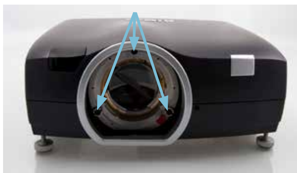
Figure 4-8. Scheimpflug Adjustment Screws
