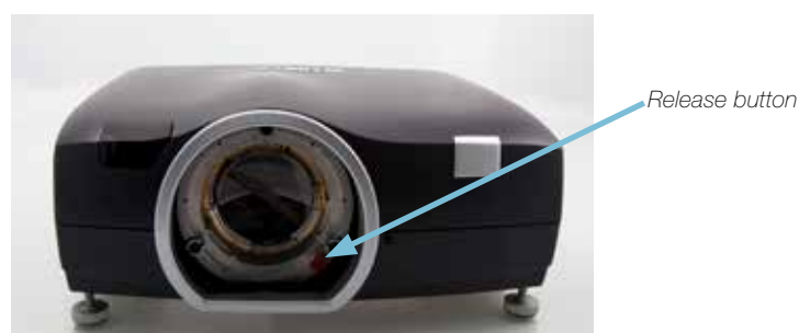
Figure 4-5. Projection lens release button
