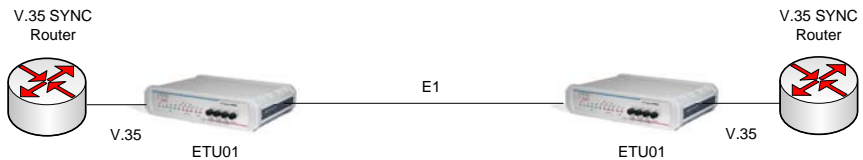
Figure 1.6 E1 Point-to-Point Application
