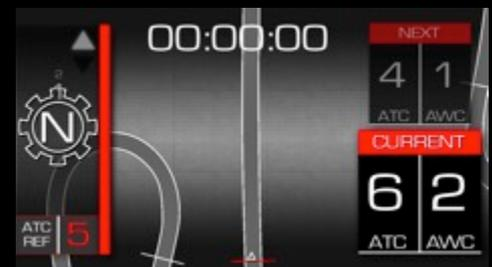
**Remarks:** the reference value for the ATC is the one selected on the bike when the system is activated. It is still possible to change it by using the ATC controls on the handlebar (+/-). The change will affect all the sectors of the track.
