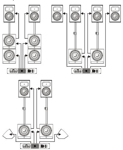
free configurable, passively and actively channelled PA systems with bass extension (left drawing) or top extension (mid drawing) or monitor extension (lower drawing) *Attention:* Please mind nominal load and impedance of the passive loudspeaker(s) you connect. For more information please contact your K.M.E. -dealer or the K.M.E. -support.
