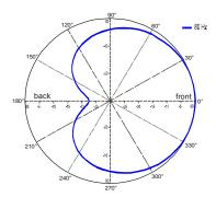
free configurable, actively channelled PA systems with directional (cardioid) dispersion in the low frequency range (lower drawing)
