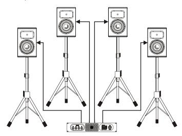
four independent and free routable channel (e.g. full-range or top units) – 4x passive top units (min. 700 W / 4 Ohm) or 8x passive top units (min. 350 W / 8 Ohm)
