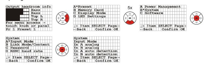
Press the marked arrow keys of the navigation-pad one after another (like shown in the scheme), to switch the input to "analogue" or "digital" or "auto detection" (by the help of the encoder). After the correct selection of the input, press the OK-button and leave the menu with the left arrow key.
