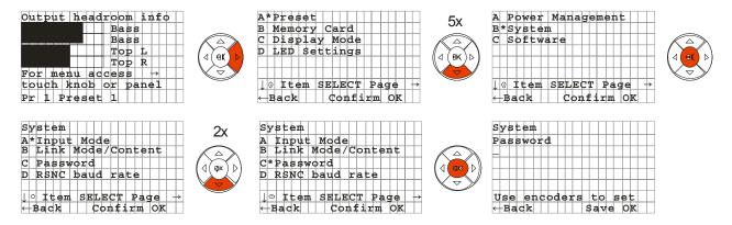
Press the marked arrow keys of the navigation pad one after another (like shown in the scheme) to open the sub menu "password". Now you can enter your password with the help of encoder A and confirm with OK. You can leave the menu by pressing the left arrow key.
