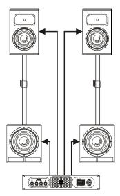
actively channelled PA system -2x or 4x top units (min. 350 W / 8 Ohm) + 2x subwoofers (min. 700 W / 4 Ohm) or 4x subwoofers (min. 400 W / 8 Ohm)
