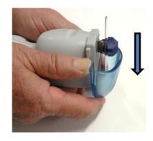
Set the nozzle back by inserting it in the guide and push down to the bottom till the automatic lock.
