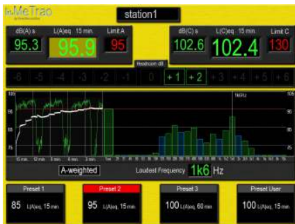
Figure 14: Yellow screen: The sound level is in the range of +1 to -1 dB from the set limit. The weighting will show whether this is for the A- or the C-weighting. If the screen is blinking yellow it means that one is recovering from being over the limit.
