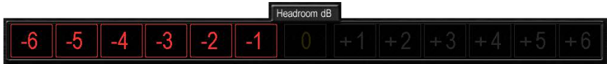
Figure 8: -6dB Headroom: The sound level is too high, the user should lower it by at least 6dB to get under the limit again
