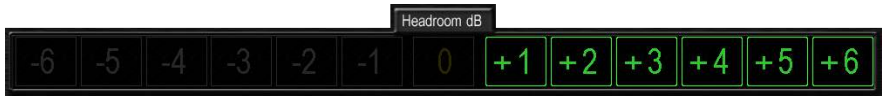
Figure 7: +6dB Headroom: The user has an extra 6dB margin to raise the sound level
