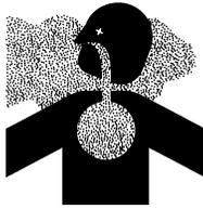
*Wear an N-100 type safety filter mask or equivalent to avoid prolonged breathing of desiccant dust. Wear safety goggles and gloves to avoid contact with eyes and skin.*
