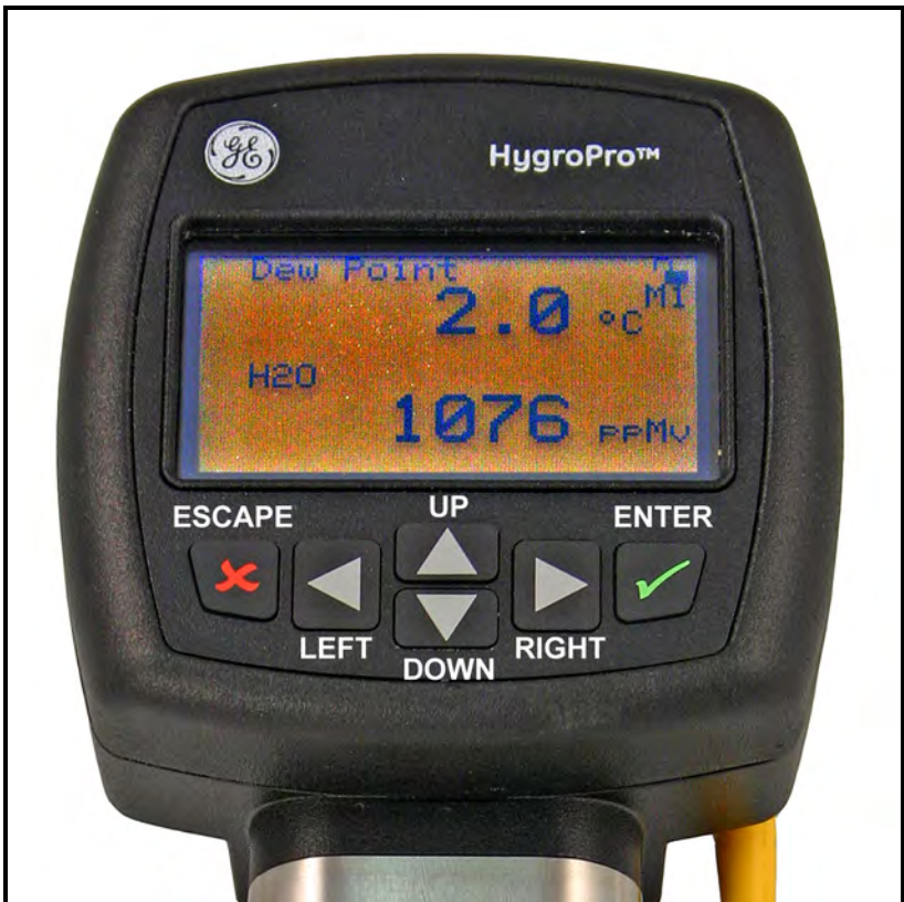
Figure 7: HygroPro Display and Keypad
