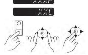
Use the product keys to enter a new offset temperature. To change from negative to positive use the left and right arrow keys. Press the P key.
