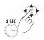
**Enter System Programming Mode** Press and hold the P key for 3 seconds.
