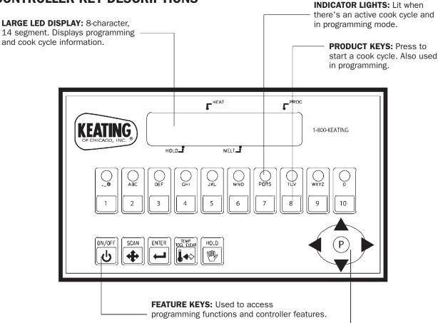
**PROGRAMMING CENTER:** Easy, cell phone-like programming. Access programming mode and change cooking parameters.
