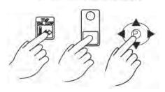
**Set Cook Time** Actual set time will be displayed. To change, press toggle clear to change the time to zero. Type in a new time using the product keys. Press the P key.
