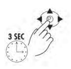
**Enter Offset Programming Mode** Press and hold the P key for 3 seconds.
