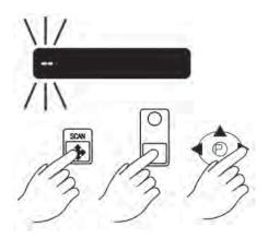
A flashing dash will be displayed. Press the SCAN key and use the product keys to spell a new word. Press the right arrow key to advance to the next character position.
