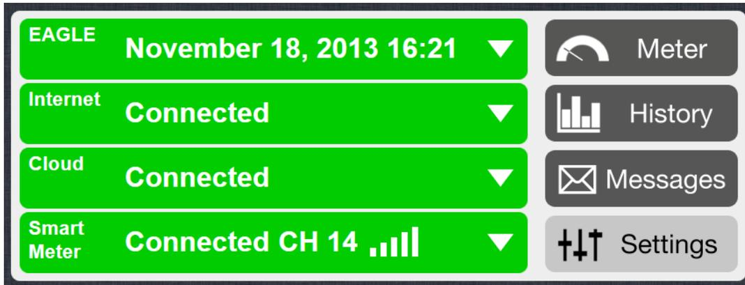
The status bars on the Settings page are color-coded to indicate status. Bars are green for normal operation, while a red color indicates an error condition and a grey bar indicates an inactive function.
