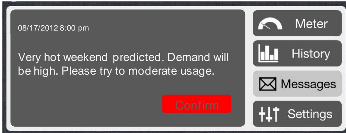
When a new text message is received from the meter, you will see the **Messages** button pulse red to indicate that there is an active message. When you click on the button the message will be displayed.
