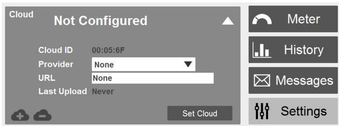
This sub-page is used to configure your **EAGLE™** to stream your real time smart meter data to an internet cloud service. Select the cloud service you want from the Cloud List drop-down menu for "Provider", and click the "Set Cloud" button at the bottom right. To complete your connection to the Cloud Service, you will also have set up an account with them. See the "Connecting to a Cloud Service" section for details
