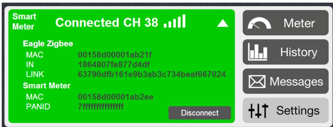
This sub-page provides information about the ZigBee wireless link between your **EAGLE™** and the smart meter. Clicking the “Disconnect” button in the lower right corner terminates the connection to the smart meter. The meter will not talk to the **EAGLE™** again until it is re-provisioned by the utility. This function can be used to move the **EAGLE™** to a different meter.
