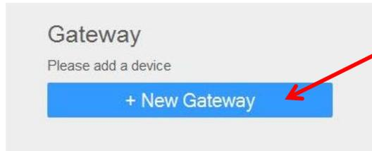
This sends you to the “Add New Gateway” page. Enter the Cloud ID and the Install Code for your **EAGLE™**. These numbers can be found on the Information Label that is on the underside of the unit.
