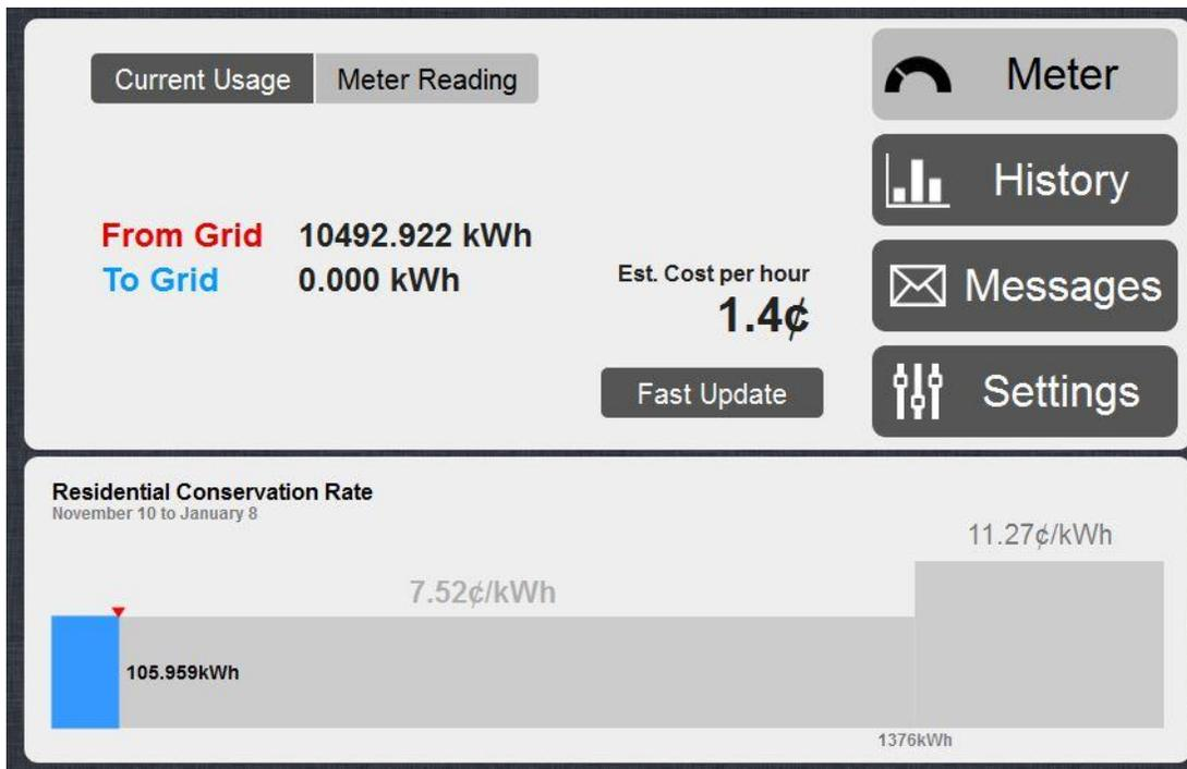
You can switch between these two modes by clicking the “Current Usage” and “Meter Reading” buttons above the usage display.
