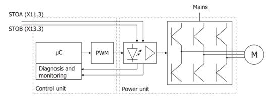
The test required for monitoring is performed by the frequency inverter automatically. If the test results negative, the frequency inverter cannot be switched on anymore. Starting is possible again only after the frequency inverter was completely disconnected from voltage supplies and error has been corrected.
