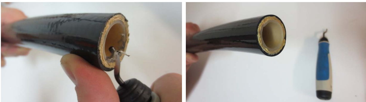
Use a proper tool to remove burrs and/or residual from the cut surface.
