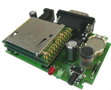
CAN Board with RTC battery
