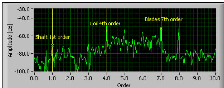
Figure 2-3. Order Spectrum With Changing Rotational Speed
