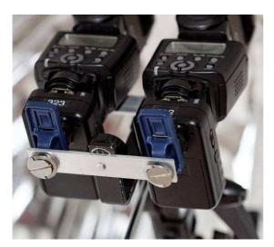
A two-flash adaptation of the single bracket. It has two cross-bars added and uses a standard umbrella swivel.
