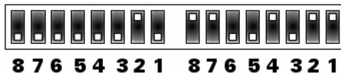
Fig. 5.10 Factory set DIL switch positions, viewed from the rear as shown in Fig. 5.9.
