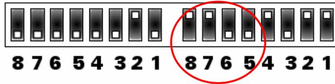
Fig. 5.13 DIL switch positions 5, 6, 7 and 8 for transmit / receive selection
