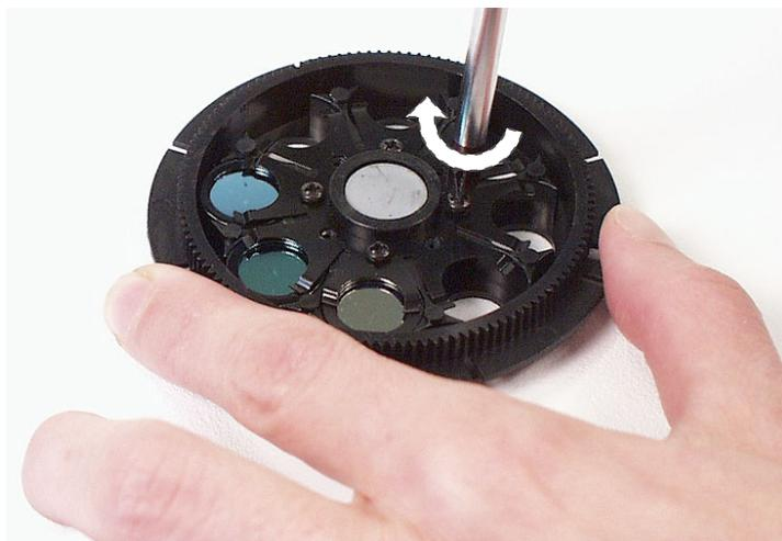
*Fig. 7.4 Removing the filter spring*
