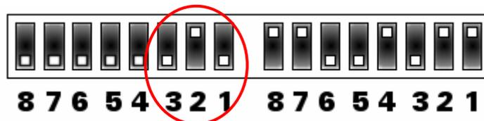
Fig. 5.14 Secondary DIL switch positions 1, 2 and 3 for Centronics type printer interface
