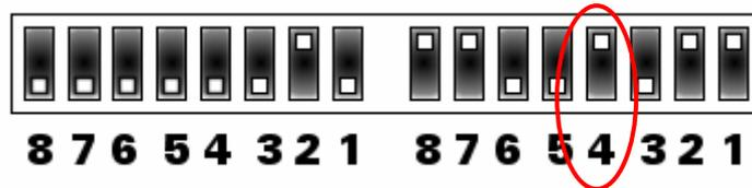
Fig. 5.12 DIL switch position 4 for handshake selection
