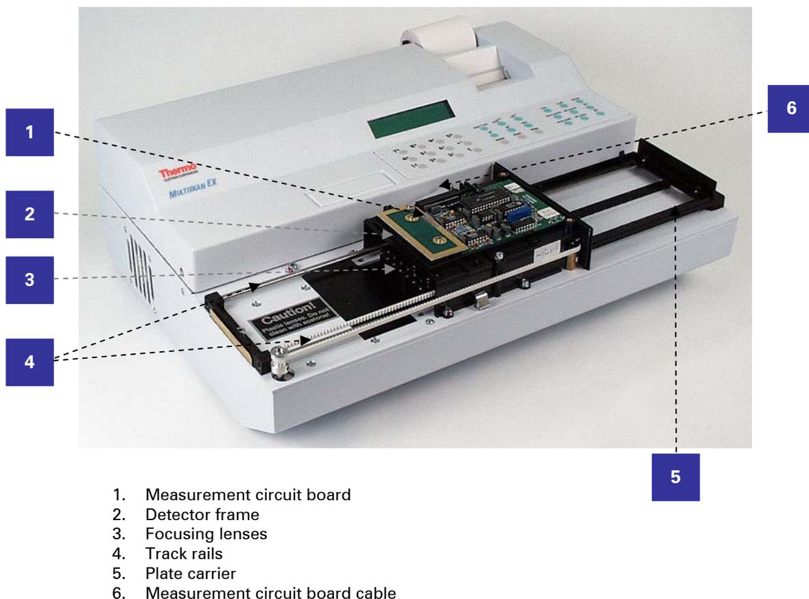
Fig. 7.1 Opening the measurement assembly cover
