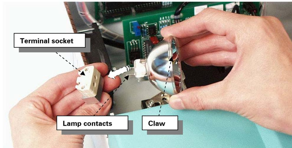
Fig. 5.6 Fitting the lamp contacts
