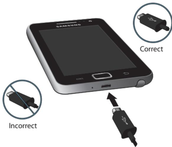
1. Plug the flat end of the Travel Charger into the Power/Accessory Interface connector and the other end into a standard AC wall outlet.
