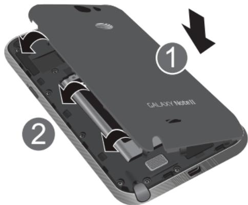
2. Press along the edge of the back cover (3) until you have a secure seal.
