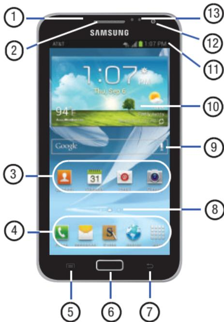
1. **Status light:** displays red when charging, green when fully charged, blue when powering up, and orange when a notification has arrived.
