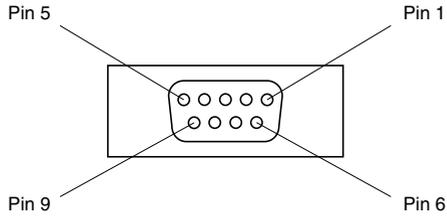
**Figure 3: 9-Pin SUB-D Connector on the Communication Card**
