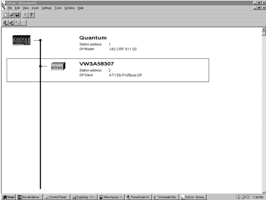
**Figure 11: Two-Module Network on SyCon Software**
