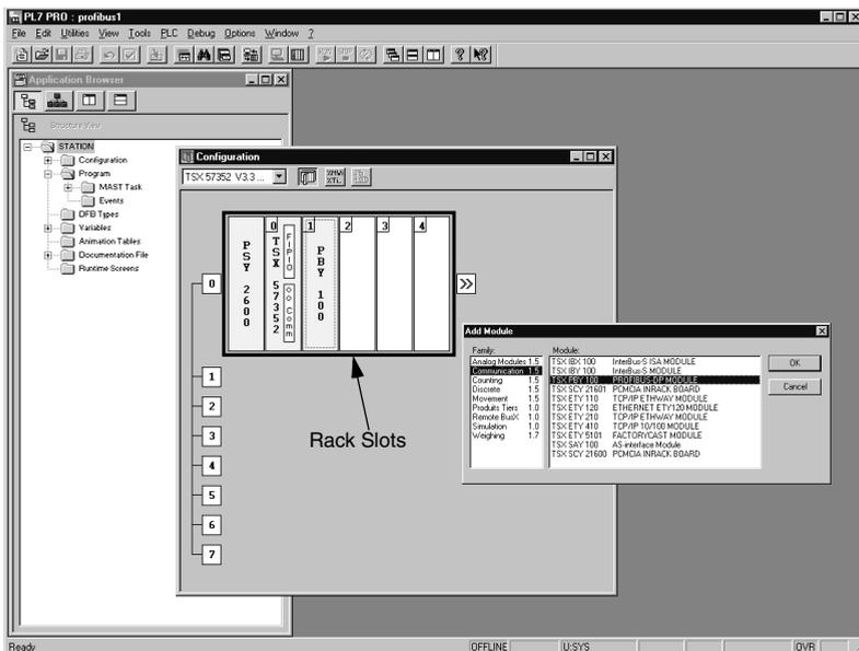
Figure 16: Adding a PROFIBUS DP Module to the Rack Configuration
