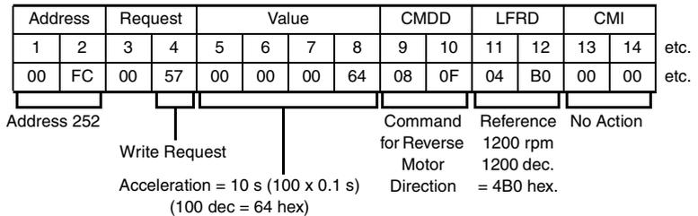
A positive response to this write request returns identical values in the first eight bytes (aperiodic, PKW, section) of the returned frame.
