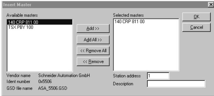
**Figure 7: Selecting a Master Module for the Network**
