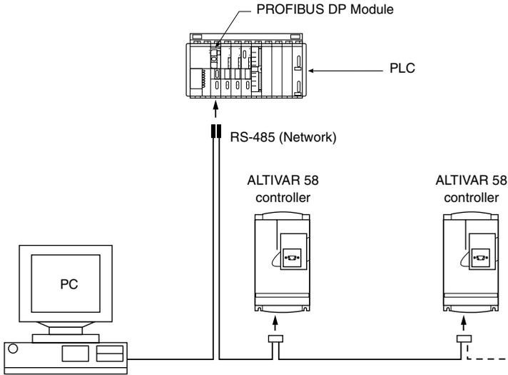
**Figure 6: Example of the Network Connection**
