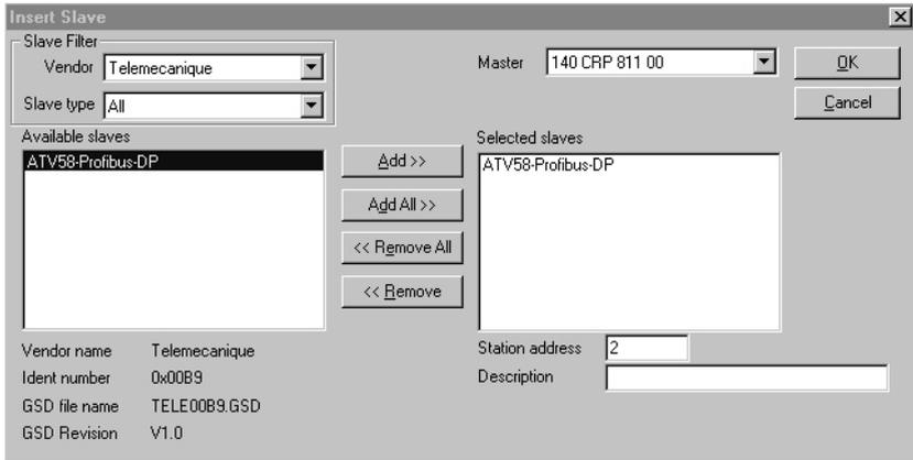
**Figure 9: Insert Slave (Module) Dialog Box**
