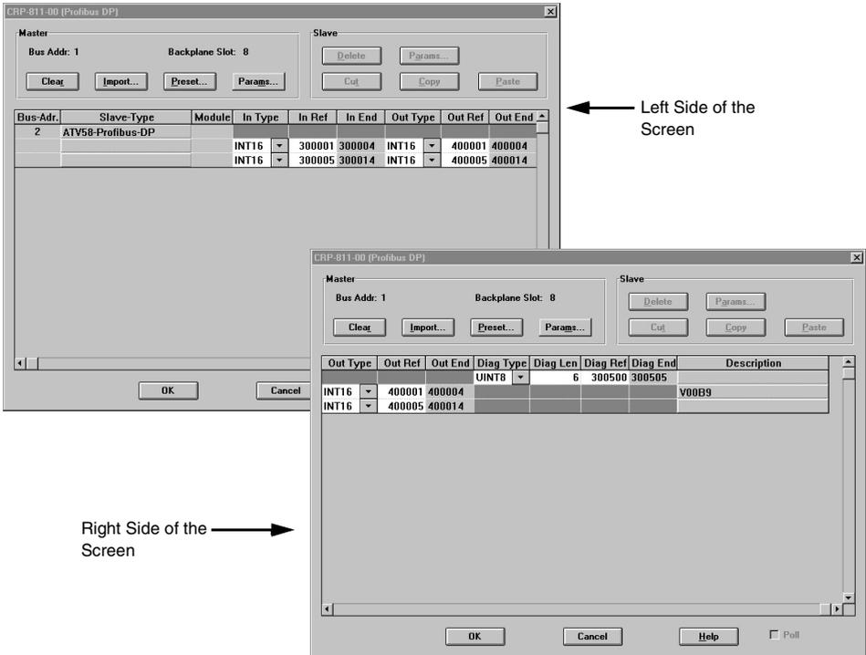
**Figure 14: Assigning Registers for PROFIBUS DP Parameters**
