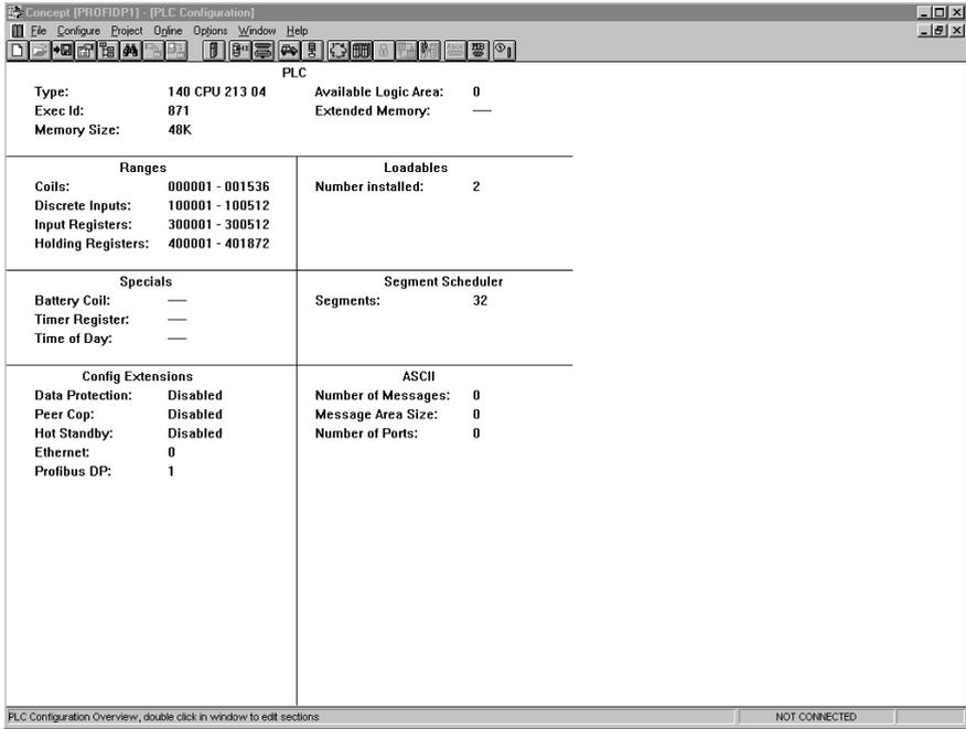
**Figure 12: PLC Configuration Window**
