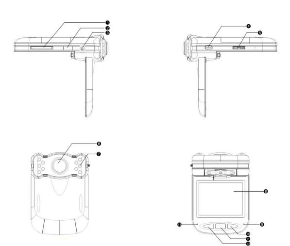
① SD Groove ② Remote Control Reception ③ AV-OUT ④ USB Interface ⑤ MENU/UP/DOWN ⑥ Red Indicator ⑦ Camera ⑧ Blue Indicator ⑨ MODE
