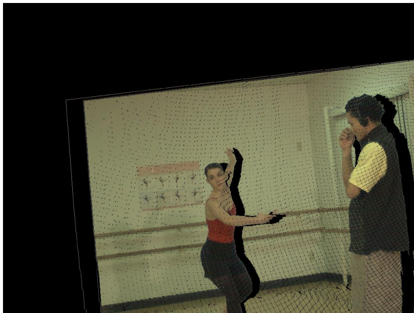
Figure 8.8: Projected Image from Camera 1 with Pitch and Yaw Rotation
