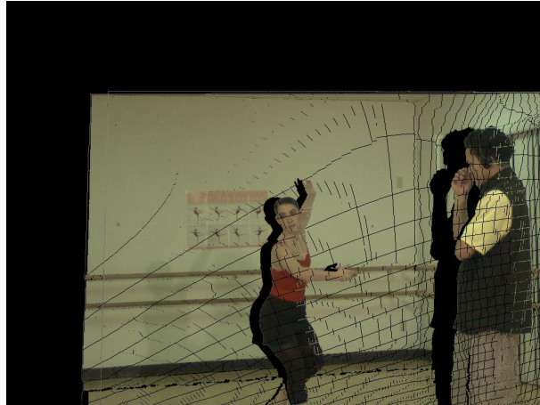
Figure 8.3: Projected Image from Camera 2 with Pitch and Yaw Rotation
