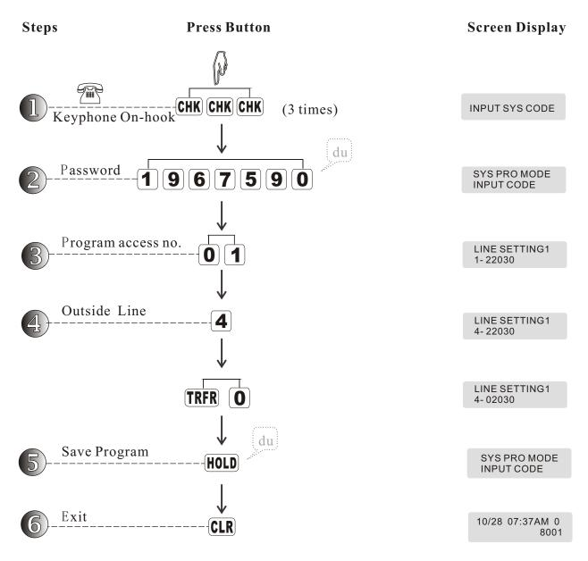
LINE1~2 is factorily open (display -22030) Program by Regular phone: Extension Off-hook+ #787-1967590 -01-4 \* 02030 # - on-hook
