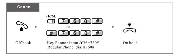
The PBX should be in intercom status when pick up handset;
