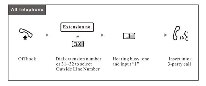
$3X: X=1\sim2$ , to use this code to select the Outside Line; You can not insert into an Intercom conversation;
