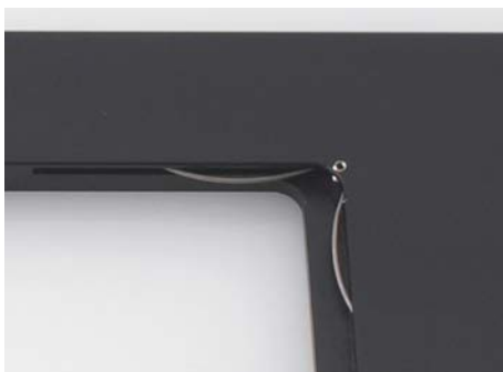
Figure 10: M-687.UN: Clip spring in clear aperture of the adapter plate
