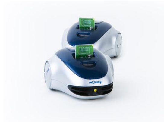
Image 14. RF modules into expansion connector.
