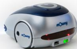
Image 16. Brake LED location. Switch on green LED.
