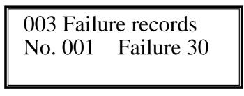
When a failure occurs, the control system will automatically inspect and judge the type of failure, and save the information with the time the failure occurs for later inquiry by maintenance personnel. It can save 100 records of failure at most. Press UP or DOWN to turn over the pages of records of failure history.
