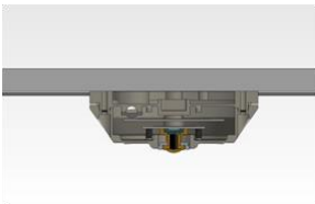
Fig1. Cross section of Surface-mount installation
