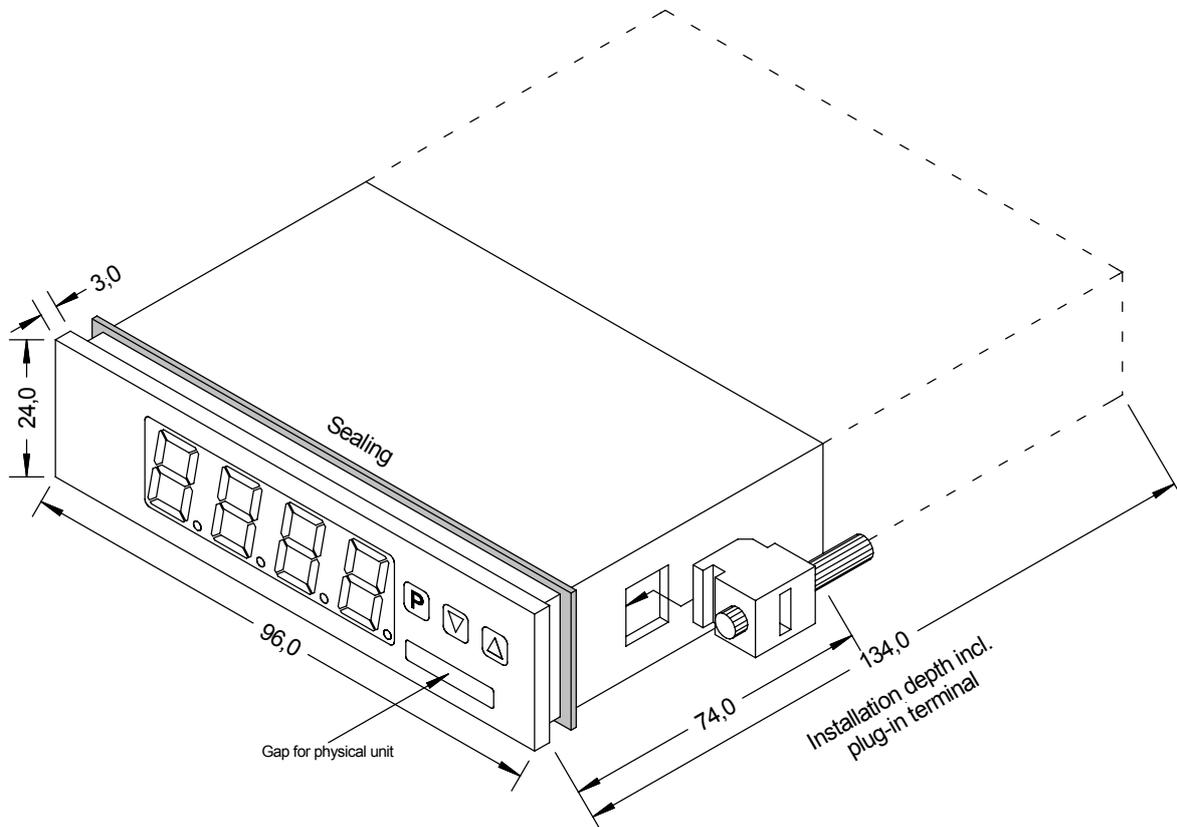
1. After removing the fixing elements, insert the device.
