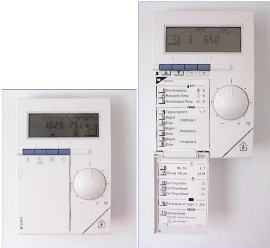
Figure 1: A heating controller and its programming interface.
