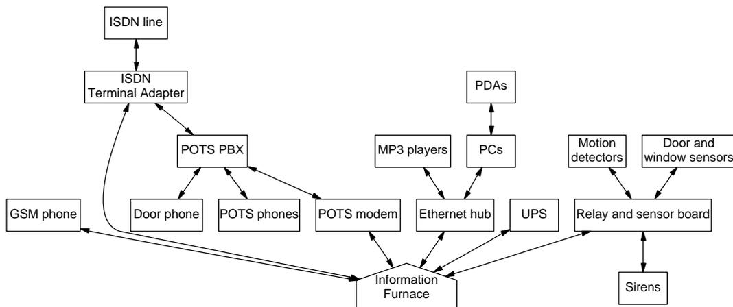
Figure 3: Information furnace connection diagram.
