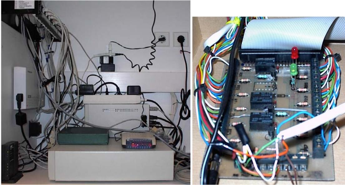
Figure 4: The information furnace (left) and the sensor connection PCB (right).
