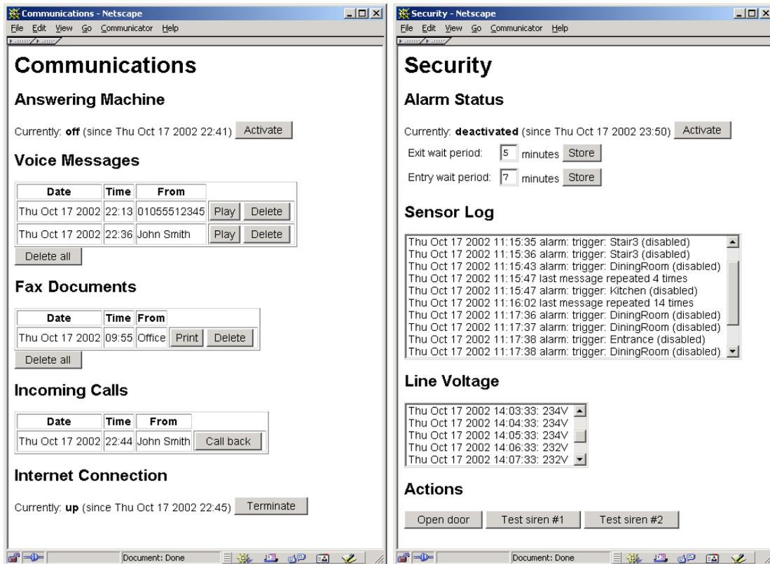
Figure 8: Web-based interface to communications and security functions.
