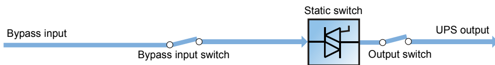
Figure 1-10 Schematic diagram of bypass mode
