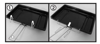
Replace screw and washers and ensure that they are fully tightened up. For a detachable handle remove screw and washers from the grill pan and keep safe.
