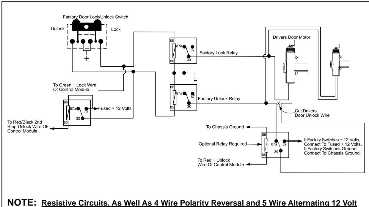
**NOTE: Resistive Circuits, As Well As 4 Wire Polarity Reversal and 5 Wire Alternating 12 Volt Door Lock Control Circuits**
