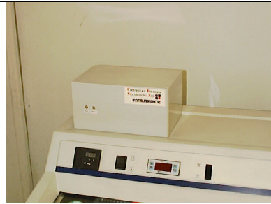
02 Place ECU on top left corner of cryostat
