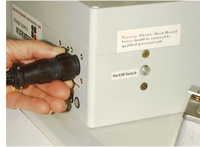
12 Connect Mech, Oil Bath Cables to ECU & Power cord to the ECU and wall outlet Turn the ECU on
