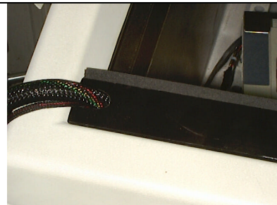
09 Place door bar with cables onto front chamber ledge. If required attach Door Bar Support Strip underneath door bar
