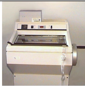
14 External-Installation Complete Cryo-Vac Shown
