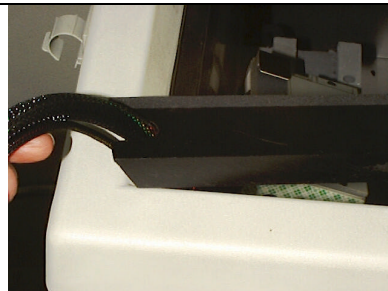
08 Route cables in door bar
