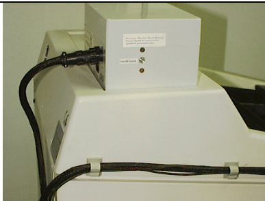
13 Mech Cable connected to ECU
