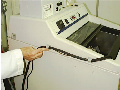
10 Adhere Cable holders along cryostat top outer wall
