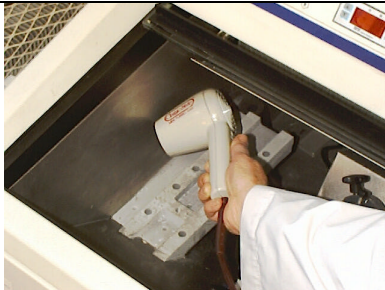
04 Heat left wall for Mech & Oil Bath placement
