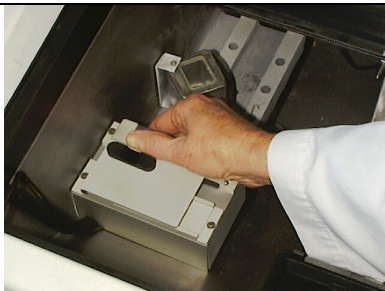
*07 Place Mech in Chamber. Place Mech low in chamber near the front wall. (Placement near the freeze bar is ideal in most cryostats)
