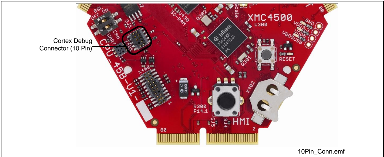
Figure 12 Cortex Debug Connector (10-pin) Layout
