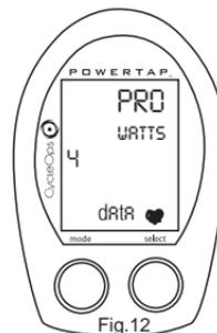
Press select to choose autostart control by heart rate (fig.12). This will allow trip time to count as long as heart rate is registered. This function is useful for transitioning from cycling to running and vice versa.
