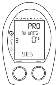
Press select button to select YES or NO for zeros included in averaging of watts. Press mode button to save.
