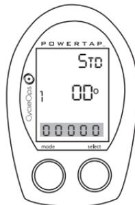
Press select button to select starting Odometer reading.
