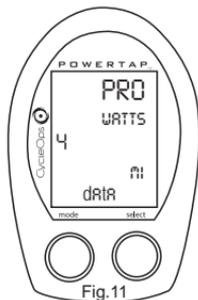
Press select to choose autostart control by speed (fig. 11). This will allow trip time to count whenever wheel speed is registering. If speed is not registering trip time will stop after 3 seconds.
