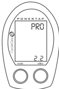
2. To enter the set up main menu hold down both buttons until the main menu is displayed
