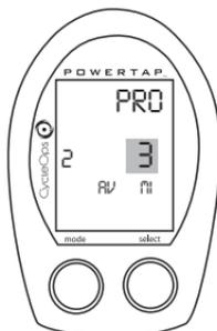
Press select button to set rate of display for speed. (rolling average) Press mode button to save.
