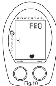
Push select until display looks like fig. 10 for heart rate only function. When this is in use all that will be displayed is current heart rate, average heart rate, trip time and time of day.
