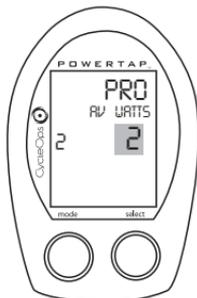
Press select button to set rate of display for watts. (rolling average) Press mode button to save.
