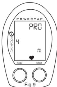
Figure 9 illustrates cycle computer only mode. This mode requires a wheel magnet on a non-PowerTap rear wheel. Align the magnet towards the bottom edge of the receiver so that it passes within 3mm of the receiver.
