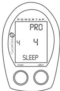
Press select to set how many minutes the CPU will stay "awake" after not receiving a valid speed or heart rate signal.
