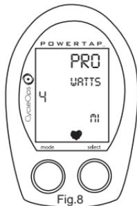
The PowerTap Pro allows you to use the unit as a cycle computer or heart rate monitor only. Fig. 8 illustrates the Power Meter Mode. Press mode to leave in this setting. Push select to change to cycle computer mode.
